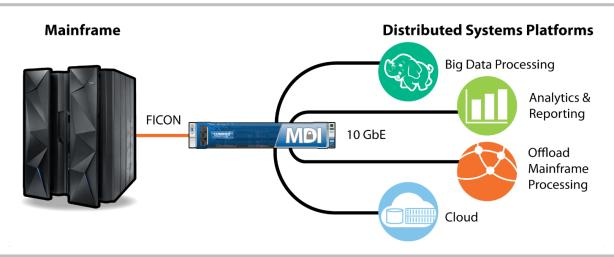
Depending on the use case, MDI Platforms can be configured with a disk cache using internal storage, or it can use dedicated or shared external storage.
