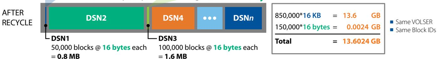
MVThsm replaces 16 KB blocks of expired datasets with 16 byte blocks, reducing space used by expired datasets by 99.9%. This enables the remaining valid datasets to be referenced by the same block IDs on the same VOLSERs without updating the HSM CDS.
